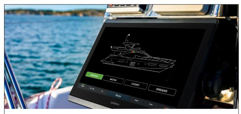
The Lopolight Control Hub appears as an app on your MFD display – the actual control hub is a device to which the individual nav lights and other equipment are connected and powered, this device has an Ethernet connection to the MFD's onboard.
